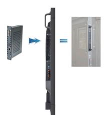
single board computer (OPS-PCAF-WS), boasts an AMD 1.6 GHz Dual Core Fusion APU and adheres
